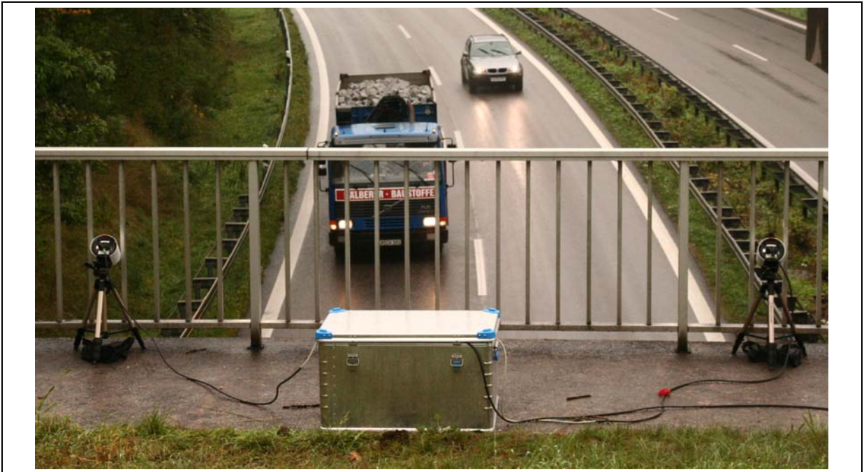
Figure 1: Two ANPR-systems set up on a bridge.
